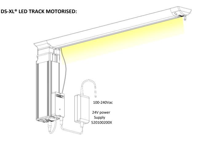
Choose the power supply according to the length of the DS-XL LED track (no difference for Shuttle S/ECO and Shuttle M):
